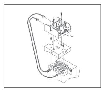
FBPC1 Fuse Block and Finger Safe Cover Kit for Field Installed Solution
